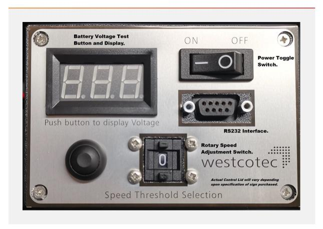
POWER TOGGLE SWITCH - SWITCHES SIGN ON/OFF
